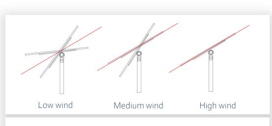
By limiting the tracking angle, we can reduce the time it takes to enter the protection state.
