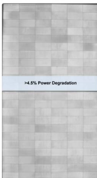
Post-PID192(-) on an almost identical BOM with 4.5% power degradation.
