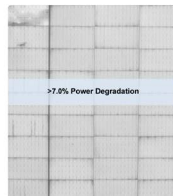
Glass//backsheet BOM post-DH2000 the module experienced >7% power loss and signs of corrosion are clearly seen around the cells' perimeters and along some bus bars.
