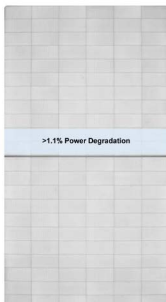
Post-PID192(-) on one BOM with 1.1% power degradation.
