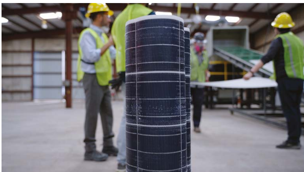
Laminate pulled from a solar panel before recycling.
