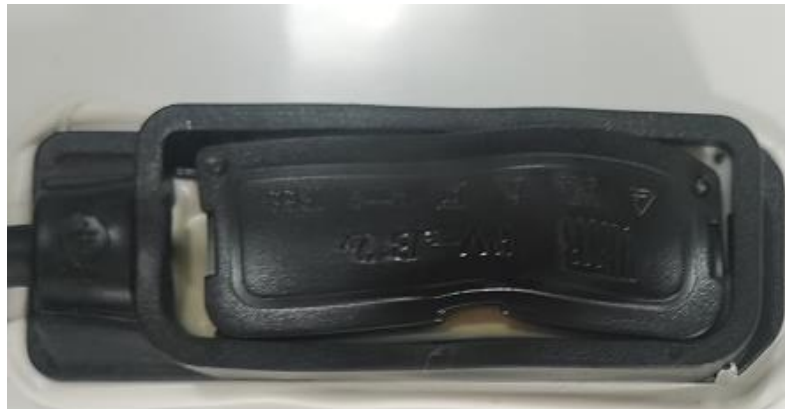
Junction box melted after RC testing
