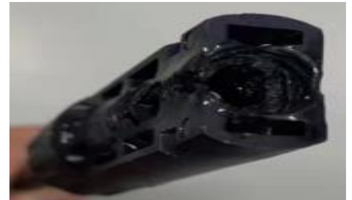
Connectors melted after TC200 and RC testing
